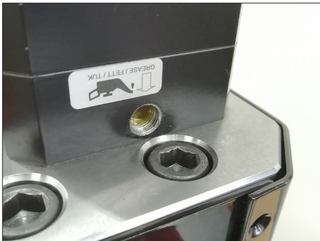
Picture 113: Threaded hole for lubrication of the servo drive
