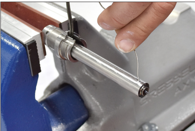
Picture 101: Installation of the new thermocouple
