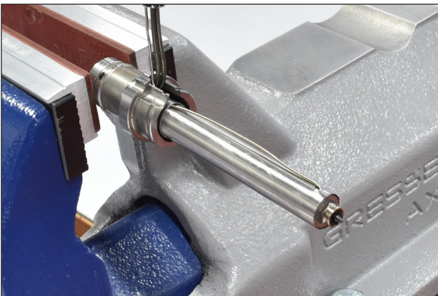
Picture 98: Pull out the protective tube
