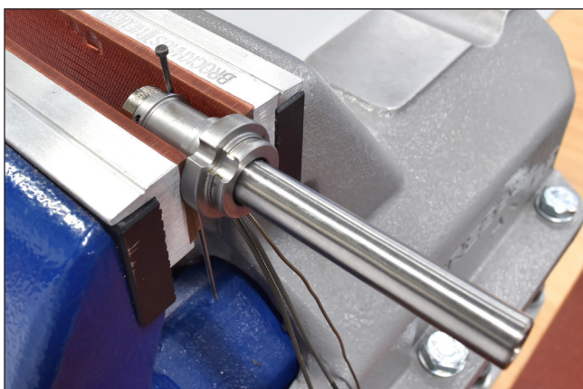
Picture 94: Pre-centre before installing the spring pins
