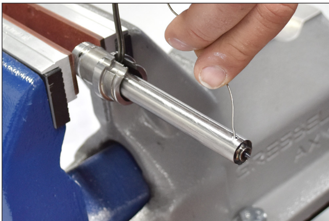
Picture 85: Installation of the new thermocouple
