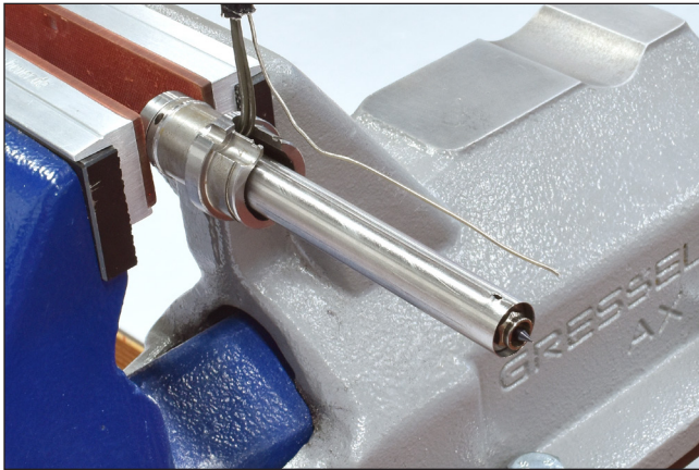
Picture 83: Disassemble the broken thermocouple
