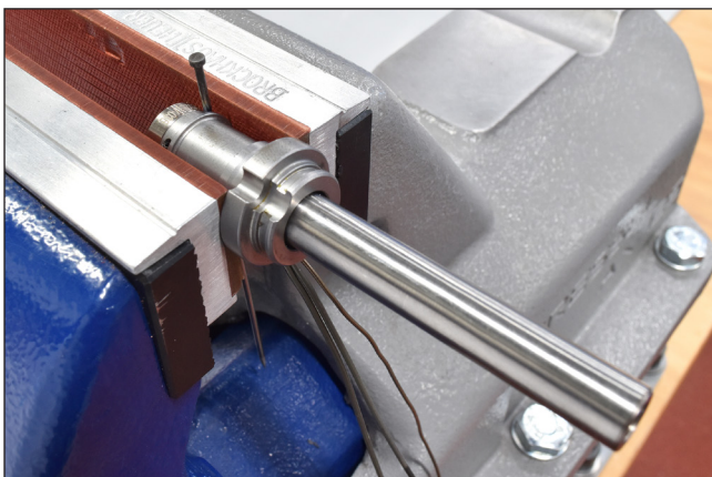
Picture 78: Pre-centre before installing the spring pins
