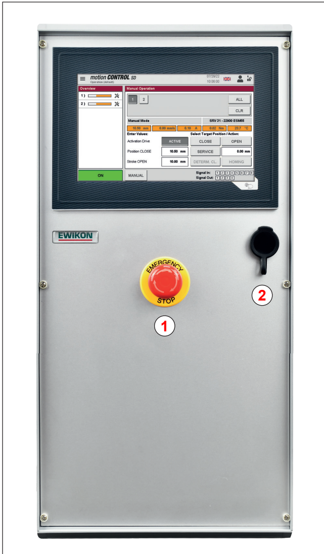
Picture 6: Connections on the front side
