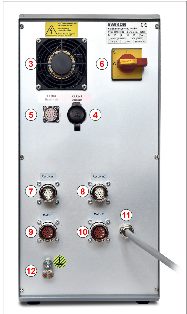
Picture 7: Connections on the rear side
